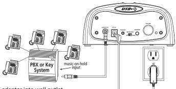
1 Plug AC adapter into wall outlet.
